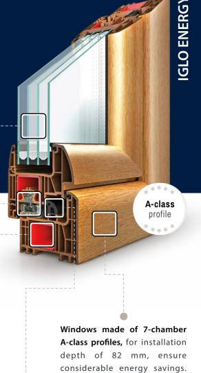
The window equipped with a system of triple sealing: external, internal made of EPDM, and central made of foamed EPDM, which guarantees high energy efficiency, and the thermal transmittance coefficient is 0,6 W/(m<sup>2</sup>K)\*. Additionally, as a standard the window is equipped with a five-chamber under-sill board with an internal gasket that increases the window tightness and improves its parameters regarding thermal insulation.
