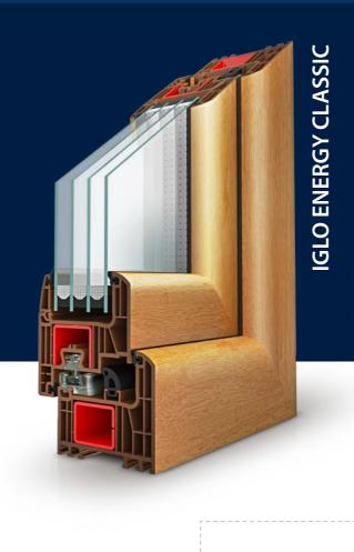
Application of glass with low-emission coatings of thermal transmittance coefficient even at Ug=0,3 W/(m²K) level ensures higher energy efficiency. The unique parameters are also obtained thanks to the use of krypton to fill the space between the glass panes.
